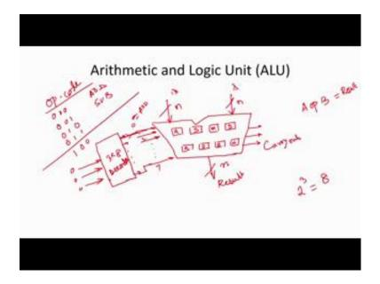
So, now just see that how we are going to construct it. Now if I say that this is the ALU I am having these 2 input and input n bit input and, say this is basically I can say that this is A, this is B and here I am going to get n bit result and say that I am having those particular processing element these are the four addition, subtraction, multiplication and division similarly 4 logic operation that say AND, OR, XOR and say NOT.
